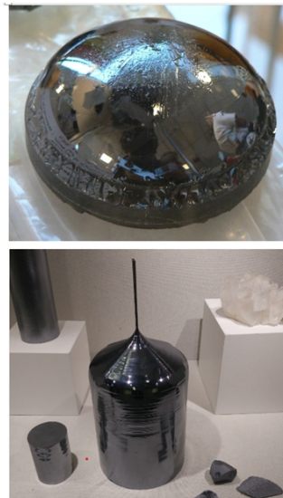
Exhibit 6: Silicon ingot (lower) and silicon carbide boule (lower)
