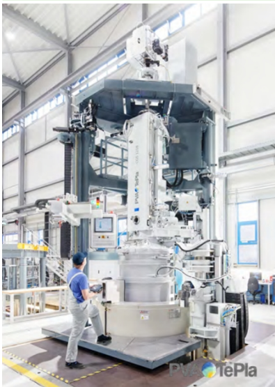
Exhibit 5: PVA TePla Si crystal puller
