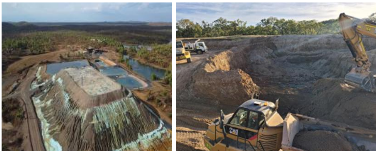
Tartana Copper Sulphate Project heap leach pad & ponds; and mining the pit fill. Source: Tartana
