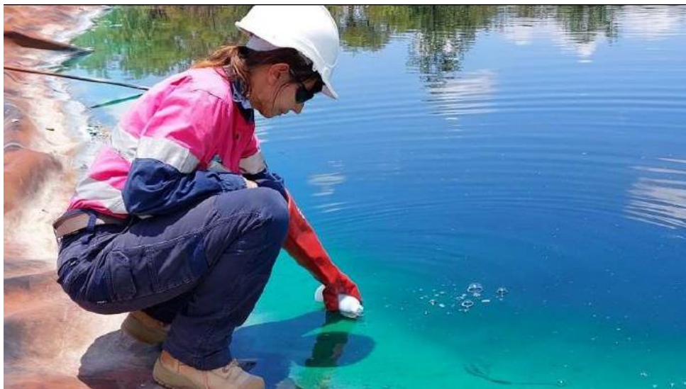
Tartana Copper Sulphate project - Sampling the process pond. Source: Tartana
