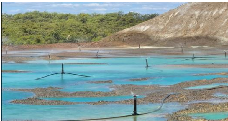
Sprinklers operating on the lower heap & copper sulphate being transported. Source: Tartana
