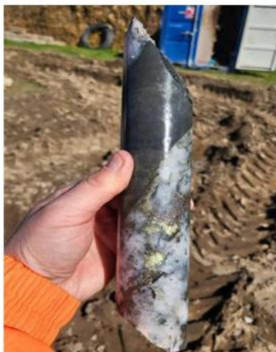
Figure 1: Example of coarse wolframite (tungsten) minerals and chalcopyrite (copper) mineralised exploration drill core from drill hole CRD036, as logged and sampled by CRL geologists. The core photograph shown is a selected example of logged drill core and is not necessarily representative of all mineralisation encountered.
