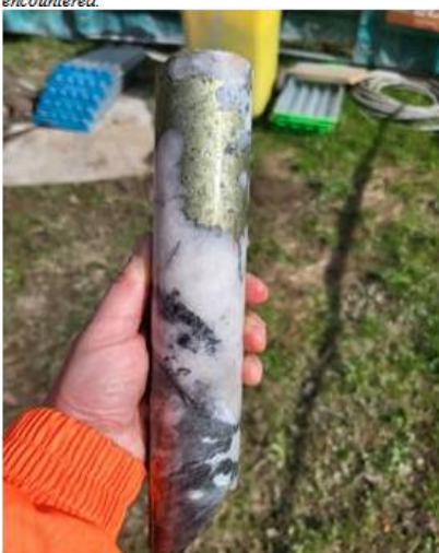
Figure 3: Example of coarse wolframite (tungsten) minerals and chalcopyrite (copper) mineralised exploration drill core from drill hole CRD037. The core photograph shown is a selected example of logged drill core and is not necessarily representative of all mineralisation encountered.
