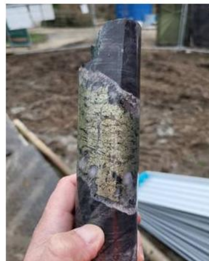
Figure 2: Example of chalcopyrite (copper) and minor cassiterite (tin) mineralised exploration drill core from drill hole CRD033, as logged and sampled by CRL geologists. The core photograph shown is a selected example of logged drill core and is not necessarily representative of all mineralisation encountered.
