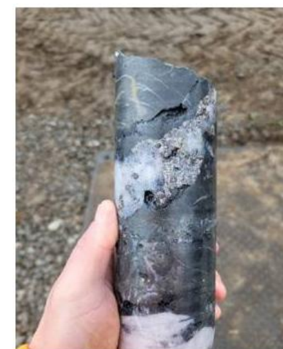
Figure 6: Example of lode-style mineralisation with quartz veins containing cassiterite (tin) and minor chalcopyrite (copper) mineralisation in exploration drill core from drill hole CRD039, outside of the Redmoor SVS. The core photograph shown is a selected example of logged drill core and is not necessarily representative of all mineralisation encountered.
