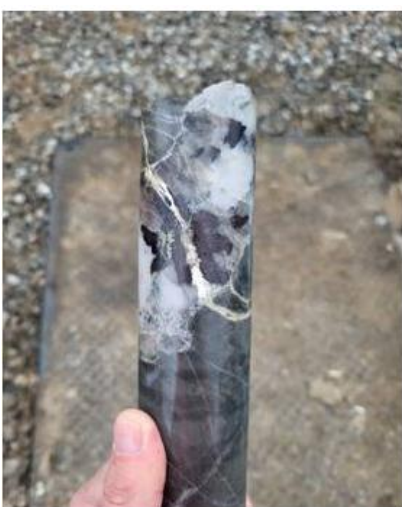
Figure 5: Example of coarse wolframite (tungsten) minerals and minor chalcopyrite (copper) mineralised exploration drill core from drill hole CRD038. The core photograph shown is a selected example of logged drill core and is not necessarily representative of all mineralisation encountered.
