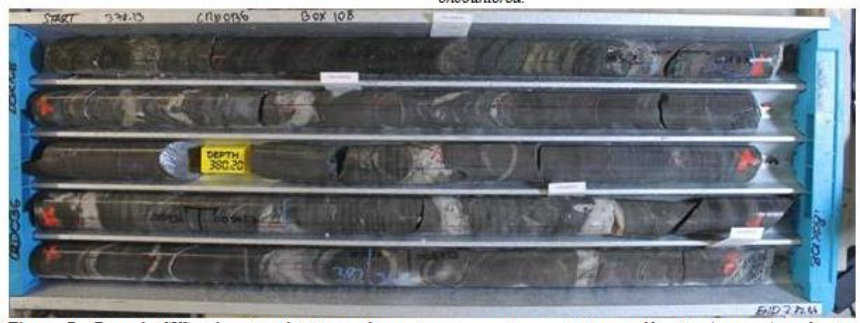
Figure 7: Example SVS-style mineralization with quartz-greisen veins containing wolframite (tungsten) and minor chalcopyrite (copper) mineralisation in exploration drill core from drill hole CRD036. The core photograph shown is a selected example of logged drill core and is not necessarily representative of all mineralisation encountered. Core is to be sampled and laboratory assays will provide quantitative results.
