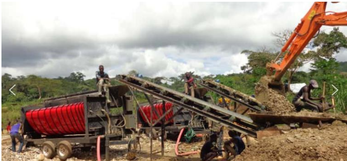
EXTRAC-TEC HPC-30 fine gold recovery system. Source: EXTRAC-TEC
