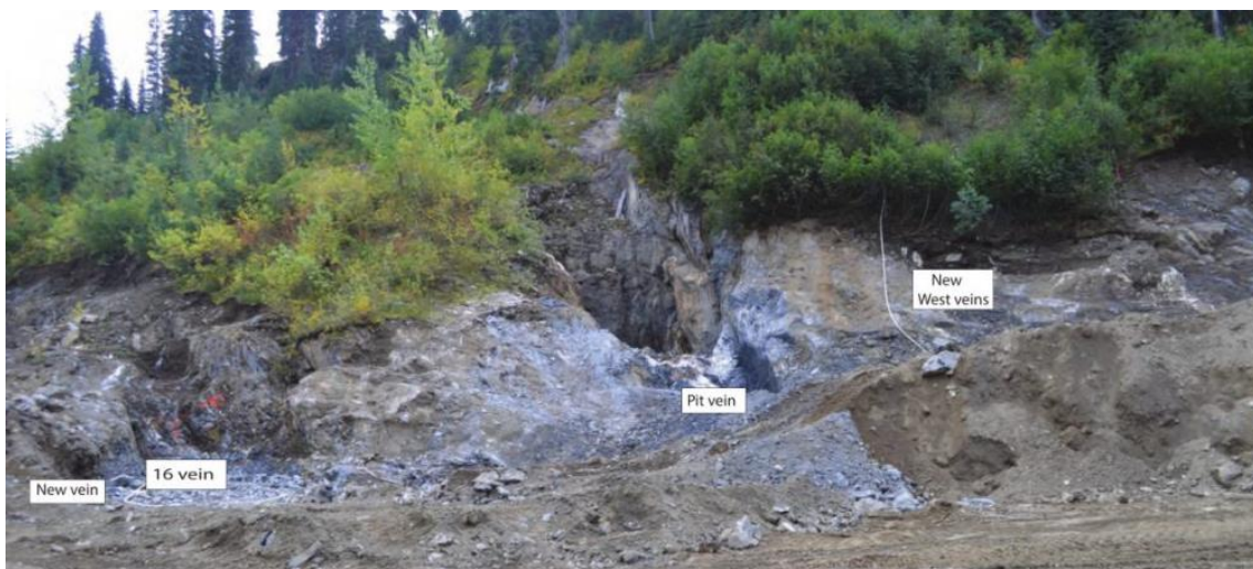
Working faces at bulk sample site (September 2025)- total width of photo is 40m. Source: Company
