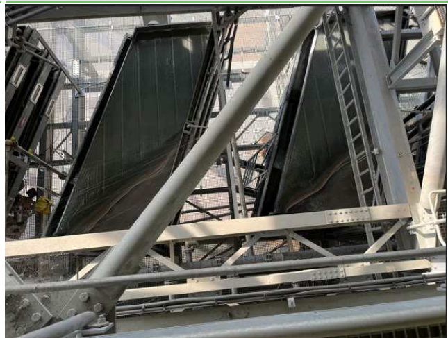
Exhibit 5: Photograph of Mpama South plant shaking tables showing pink cassiterite concentrate bands
